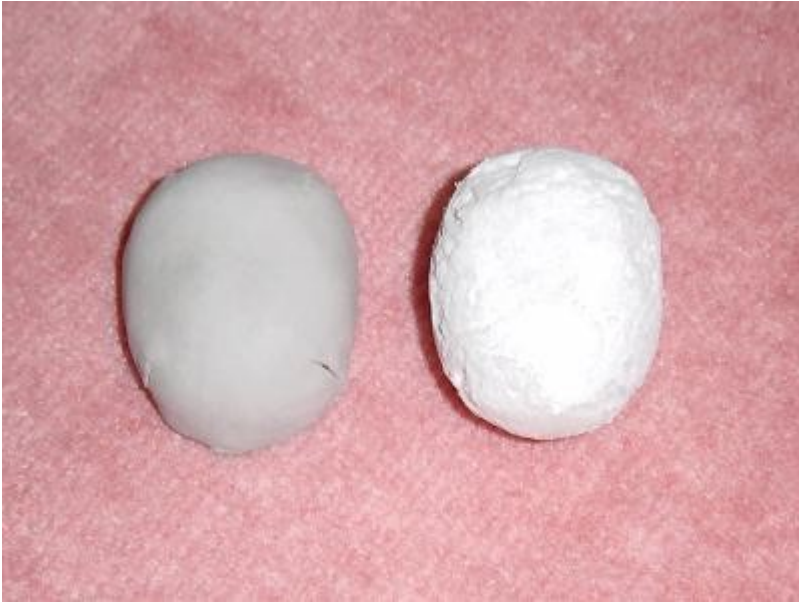
Completely dried and the clay removed from the core.
